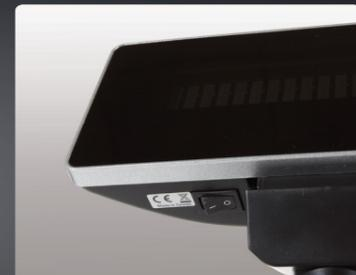
The power button is located underneath the display.
